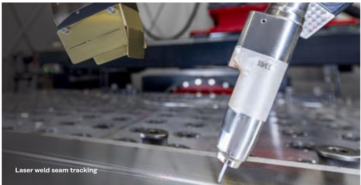
Laser weld seam tracking
