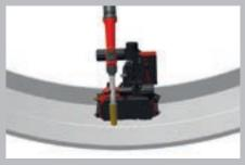
/ Welding butt welds on concave components
