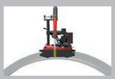
/ Welding butt welds on convex components
