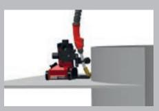
/ Welding fillet welds on convex components
