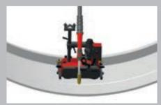
/ Welding butt welds on concave components
