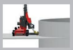
/ Welding fillet welds on convex components
